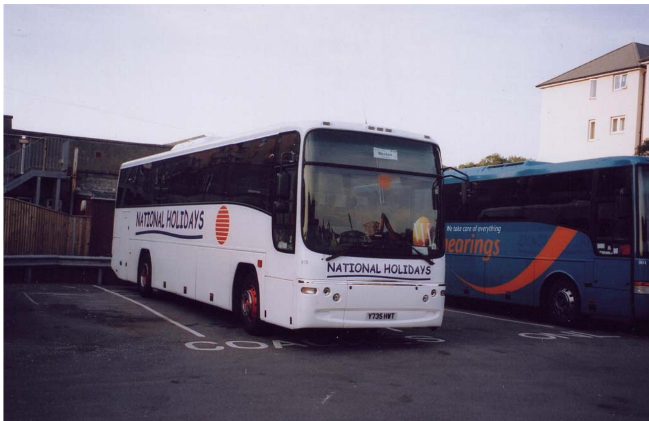
National Holidays 975 N735HWT a Volvo B10M-62 with Plaxton C49Ft bodywork at The Grand Atlantic Hotel, Weston – Super – Mare in July 2006
